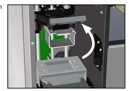
2. Pull the print platform handle (A) out from under the clamp.
