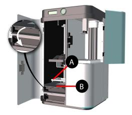
5. Carefully pull the label cover off the cartridge.
