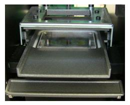
4. Rotate the material cartridge clamp lever (B) down to lower the cartridge clamp (A).
