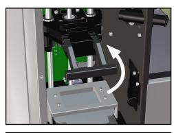
2. Insert the print platform under the clamp lever until it is seated.
