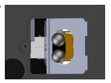
4. Carefully press the bulb base into the socket and ensure the connection is secure.
