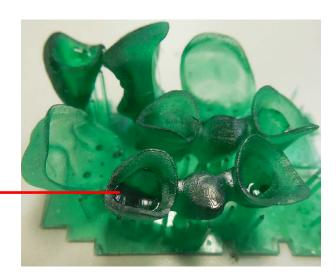
An air bubble may be trapped preventing the isopropyl alcohol from contacting the part.
