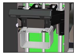
3. Rotate the print platform clamp lever down to lock the print platform.
