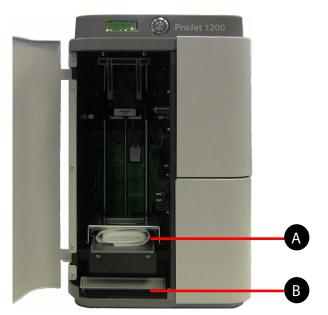
3. Loosen and remove the screw securing the bulb access panel to the bottom of the printer and remove the panel.
