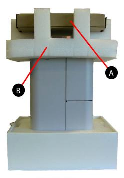
5. Carefully remove the printer from the lower boxed foam support and place it on a solid, level base where it will be used.
