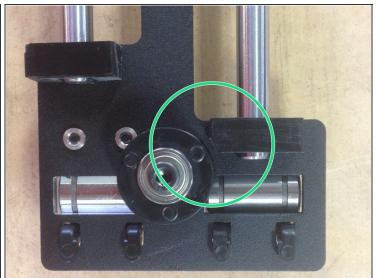
• NOTE: If you received a rod clamp with a corner cut, it is meant to be installed adjacent to the pulley, to allow the pulley to spin freely.
