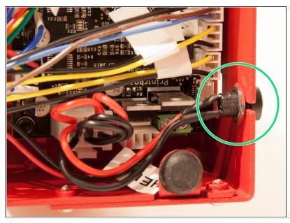
Plug the 6 pin connector of the power harness dongle into the Printrboard. The barrell connector can be attached to the base by loosening the nut off of the threads and then tightening it back down against the wiring hole of the base of the bot.
