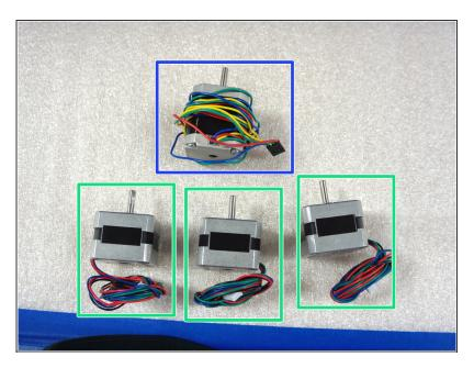
You may have received three small motors with one large motor, the large motor is only for the extruder assembly. The three smaller motors are for the X, Y, and Z axis assemblies
