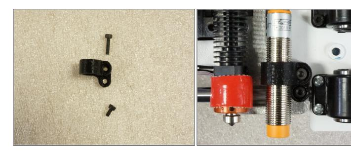
You may have received the new 3D printed sensor clamp. The sensor clamp and will need
