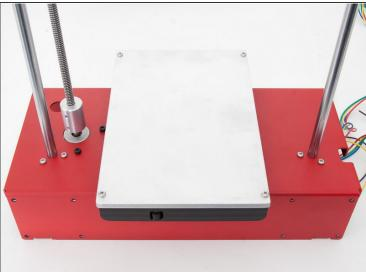
Attach the print bed with plastite screws (x4)
