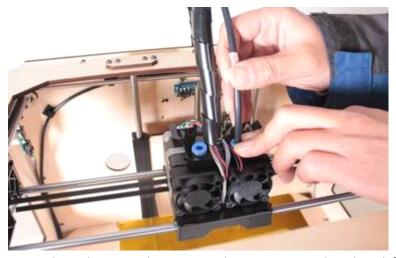
Once the tubes are disconnected, you can go ahead and feed the filament into the guide tubes from the back until you see it come out at the front.
