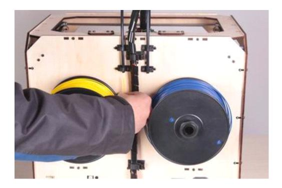
After you've fed the filament through, press the M. The machine will start to heat both extruders
