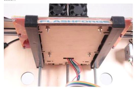
It's very important that you always move two knobs during each step -- if you try to move only one knob at a time, the script can have unexpected results. Also, make sure that you're moving the specific knobs the script is telling you to use.
