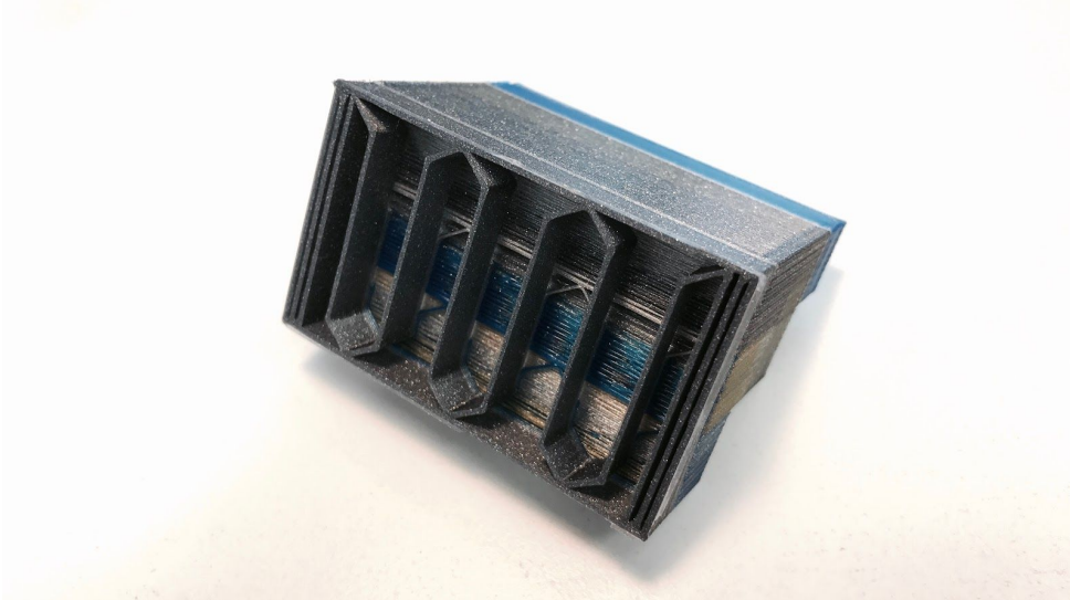
When filament change is not needed, smart wipe tower is hollow.
