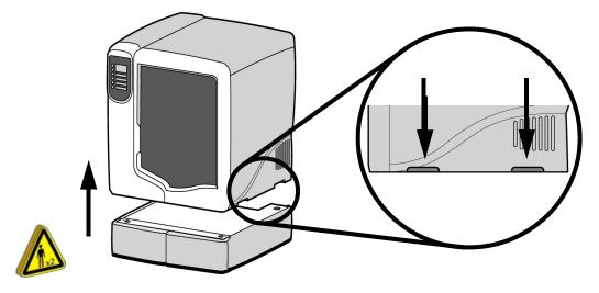
14. Position the second material bay on top of the existing material bay. Be sure the feet and pins are properly aligned. See Figure 3-3.
