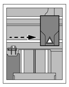
3. Remove the tip wipe assembly by lifting the assembly up and out of the printer. Discard this tip wipe assembly. See Figure 5-3.
