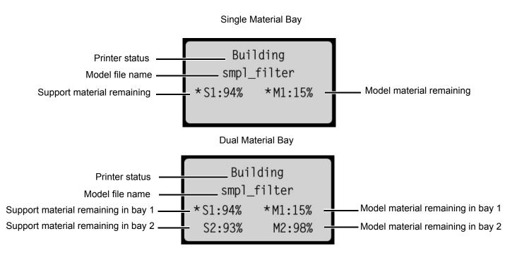
**Note:** If a material amount is flashing, it indicates that the remaining material will not be enough to complete the current build.
