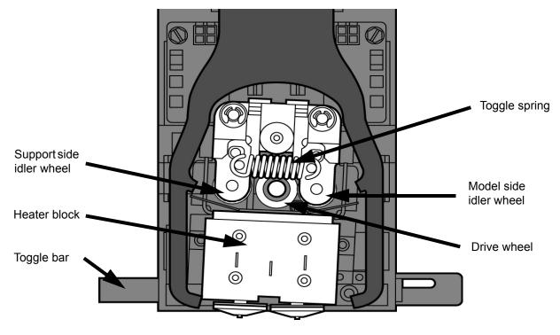
Figure 6-6: Toggle bar in neutral position
