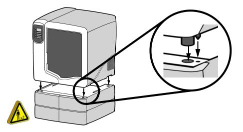
16. Remove the black plugs from the model and support Y blocks by pushing in on the coupler rings and pulling outward.
